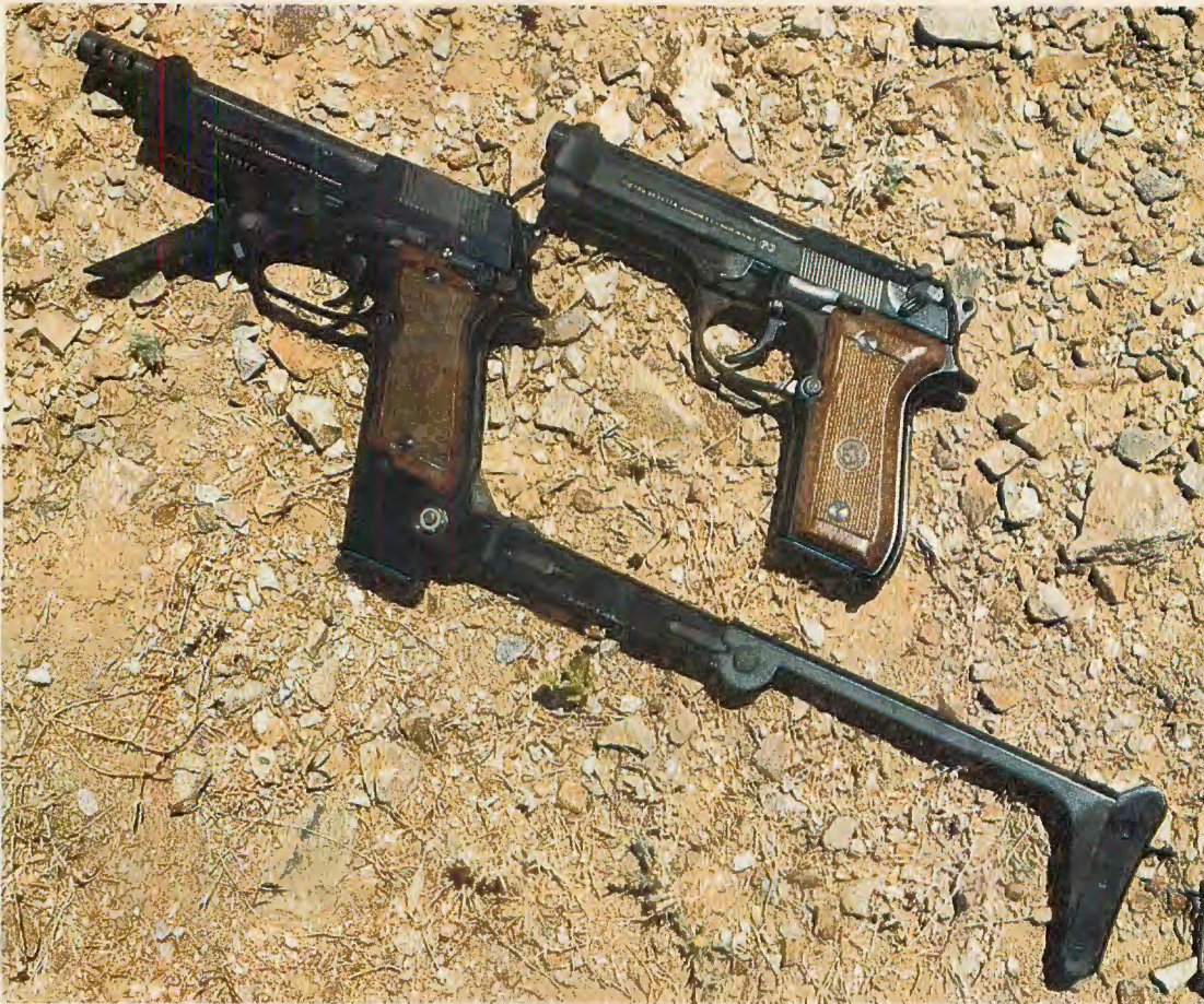
Beretta 93R machine pistol (left), with folding fore-grip extended and folding buttstock attached, shows relationship to Model 923B, its immediate antecedent.
